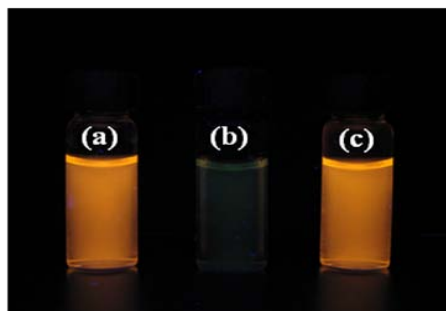
Figure 4-15. Fluorescence intensity changes of (a) PyA4 (b) PyA4 -Cu 2+ complex, and (c) PyA4 -Cu 2+ with PPI; [ PyA4 ]=10 \mu M; [Cu 2+ ]=40 \mu M; [PPI]=80 \mu M in 20 mM HEPES buffer at pH 7.5.
